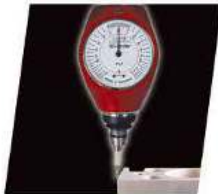
2. Zero position has been reached, spindle axis = workpiece edge: The NC-control can be set to "Zero".
